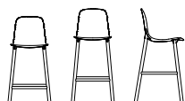
Stool with high back - wooden base L 49 P 58 H 101-111 cm W 19 2/8 " D 22 7/8 " H 39 5/8 -43 5/8 "
